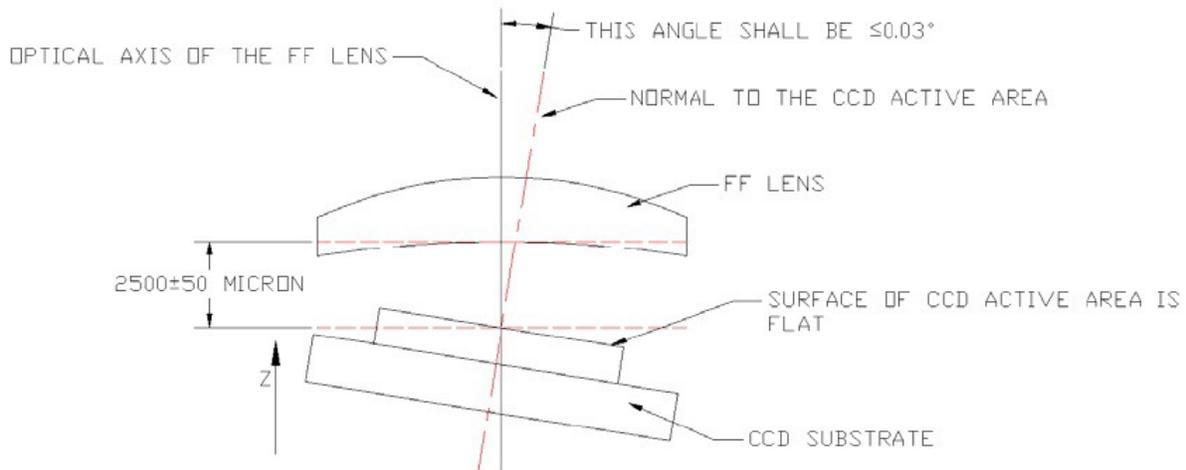
Figure 5. The alignment relationships constraining the field flattener/detector relationship.
