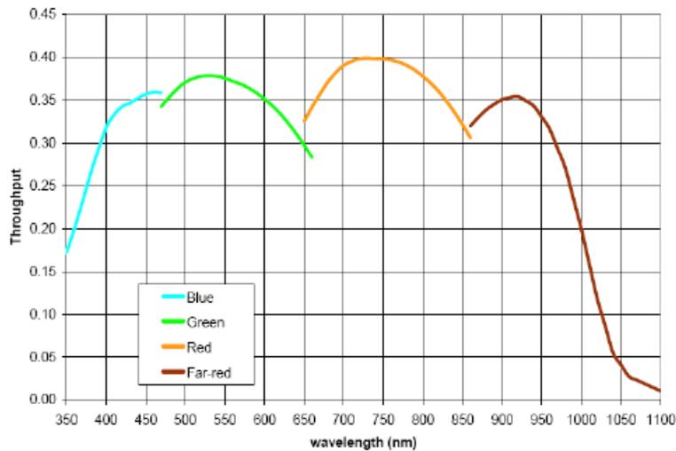
**Figure 4.** Predicted throughput of LRS2 including the IFU and spectrograph, but excluding the HET and atmosphere. The same model has been verified on sky for VIRUS-P. The exact edges of the dichroic beamsplitter bandpasses have not been included, but they will be designed to have sharp transitions at wavelengths close to 470, 620, & 830 nm.
