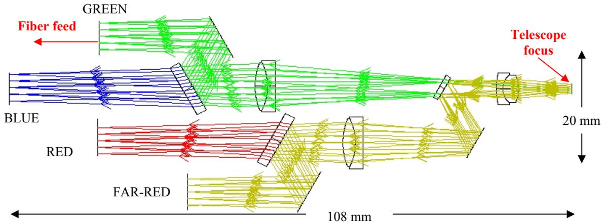
**Figure 3:** Optical Design of the IFU Feed for LRS2. Light from the input field is collimated and split into four wavelength ranges by a series of 3 dichroics. Each wavelength range is focused onto a lenslet - coupled fiber array and is transmitted to a separate spectrograph. The design is “folded-out” for clarity.
