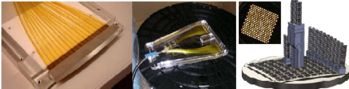
**Figure 2:** VIRUS IFU Construction. The left panel shows a slit for a single spectrograph in a production jig. The middle panel shows the double slit end of a production IFU prior to integration into its housing. The right panel shows how the input ends of the IFUs for VIRUS (only a few shown) and the feed for LRS2 at the center of the field will be integrated together to allow parallel observing. The inset shows the input end of the VIRUS-P IFU.
