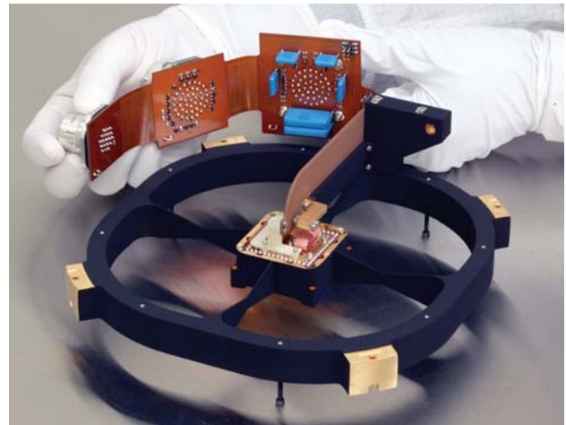
Figure 8: detector mount assembly. In this orientation, the field flattener is on the underside and the detector is facing downwards. The cold link and flex circuit for detector signals are aligned above one of the spider vanes. A blackened cap (not shown) mounts over the cold block and header board assembly, to prevent reflection light that falls on the central hub.
