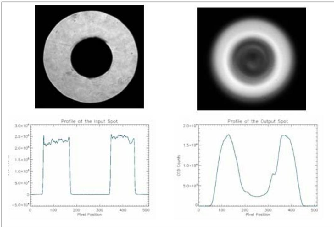
Fig. 14. An image and radial profile of both the input and output spot of our current fiber optic test bench. The central obscuration constitutes  $\sim 42\%$  of the input spot diameter and mimics the secondary mirror of the HET. The effect of FRD can be seen in the shallower radial profile of the output spot.
