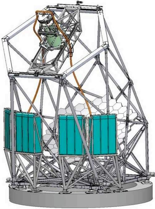
**Figure 3:** Drawing of the upgraded HET with all components, the new Tracker, PFIP, WFC. The boxes (blue-green) on the sides of the telescope house the suite of spectrographs for VIRUS. The two cables (orange) contain the fibers which run from the IFUs to the spectrographs.
